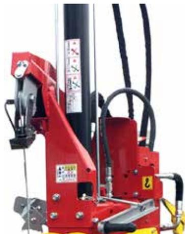
..... ● TREUIL HYDRAULIQUE AVEC REGLAGE VITESSE
