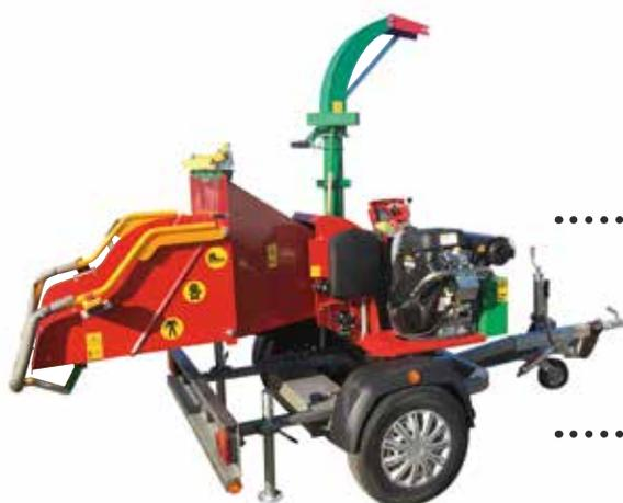
..... ● TUBE D'ÉJECTION REHAUSSÉ DE SÉRIE REPLIABLE SANS OUTILS ET ORIENTABLE 360°
